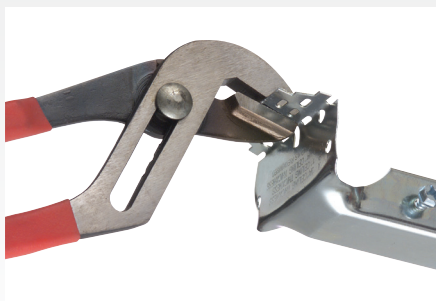
Bracket ends are pre-set for a 1/2" ceiling. For other ceiling depths, bend the bracket ends along the appropriate score line.
