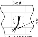
1. Cut 3-3/8" X 5-5/8' Hole in Block. Pull Wiring.
