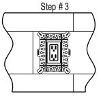
Fasten Non-Metallic Cover to Substrate. Wire Device \*
