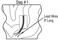
1. Cut 3-3/8" X 5-5/8" Hole in Substrate. Pull Wiring.
