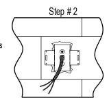
Fasten Steel DSBVM1 Box to Substrate with Masonry Fasteners. Pull Wiring thru Connector in Steel Box. (Not Provided)
