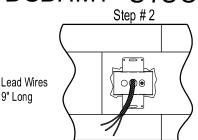
Fasten Steel DSBHM1 Box to Block with Masonry Fasteners. Pull Wiring thru Connector in Steel Box. (Not Provided)
