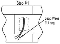
1. Cut 3-3/8" X 5-5/8" Hole in Block. Pull Wiring.
