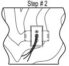
Fasten Steel DSBVS1 Box to Substrate. Pull Wiring thru Connector in Steel Box. (Not Provided)
