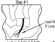
1. Cut 3-3/8" X 5-5/8" Hole in Substrate. Pull Wiring.
