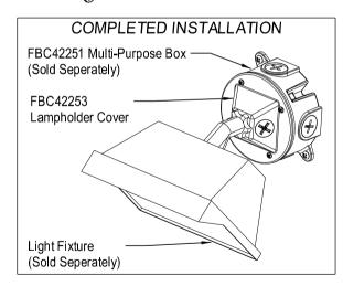
All wiring must be in accordance with National (NEC/CEC), State and Local Electrical Codes.
