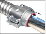
1 Simply loosen the screws and insert end stop bushing if necessary. Slip connector onto MC cable. Retighten screws on strap.
