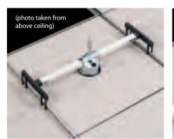
2 Place box over hole. Snap plastic ends of
