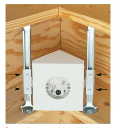
2 Loosen the screws noted above. Slide box along brackets to center it between rafters. Tighten
