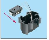
2 Pull non-metallic cable. Install in box using supplied NM94 cable connector. Wire receptacle and install in box.
