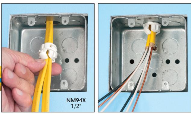
Save money with Arlington's non-metallic NM cable connectors. They're the *lowest* cost NM cable connectors on the market, and the fastest to install! Simply push the connector into the knockout, and you're done.
