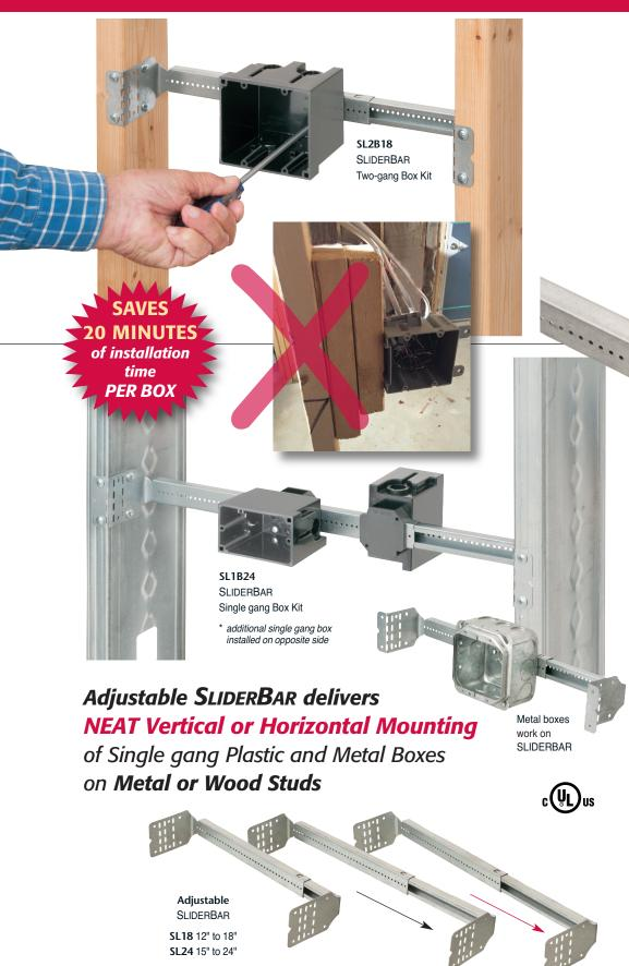
Here's the easy, NEAT way to mount single or two-gang boxes between wood *or metal studs* with non-standard spacing.
