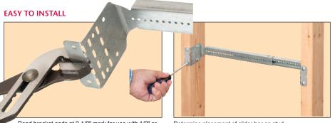
Bend bracket ends at 2-1/2" mark for use with 1/2" or 5/8" thick wall board. Ends can also be bent 90° or backwards at 180° as needed for inside mounting.
