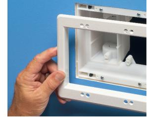
3 After wall surface is installed, wire receptacle and low voltage devices. Attach trim plate (screws provided.) Tighten mounting wing screws – if desired – for added support.
