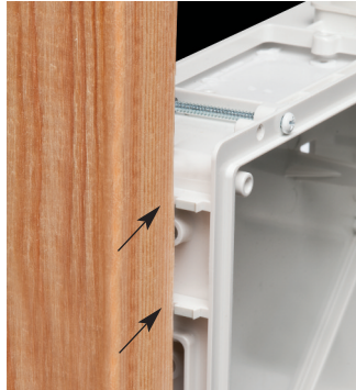
Positioning tabs are set for 1/2" or 5/8" drywall.
